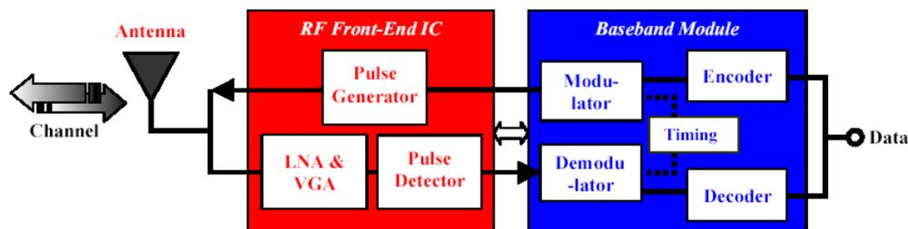
Figure 1 - Example of architecture of an UWB transceiver as considered in this project.
