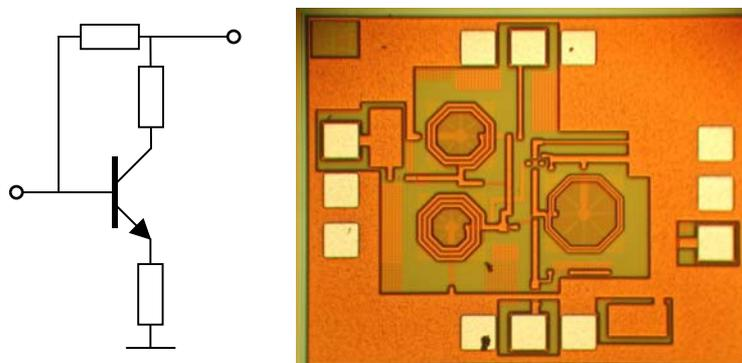
Figure 2 - Simplified AC schematics and chip photograph of the LNA (chip size: 1x 1.3 mm)
