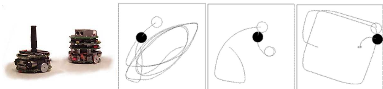
Figure 3. Co-evolutionary prey (left) and predator (right) robots. Trajectories of the two robots (prey is white, predator is black) after 20, 45, and 70 generations.
